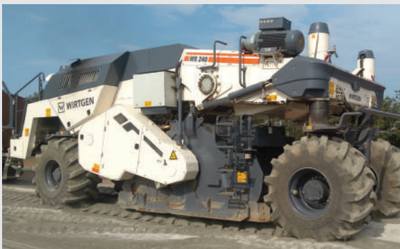
FDR in process in Uttar Pradesh with StabilRoad
